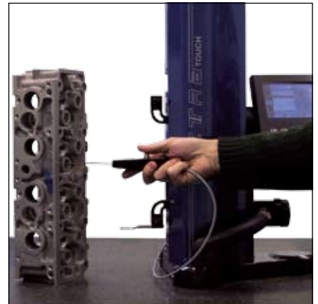
Measurement using temperature compensation system with optional external sensor
